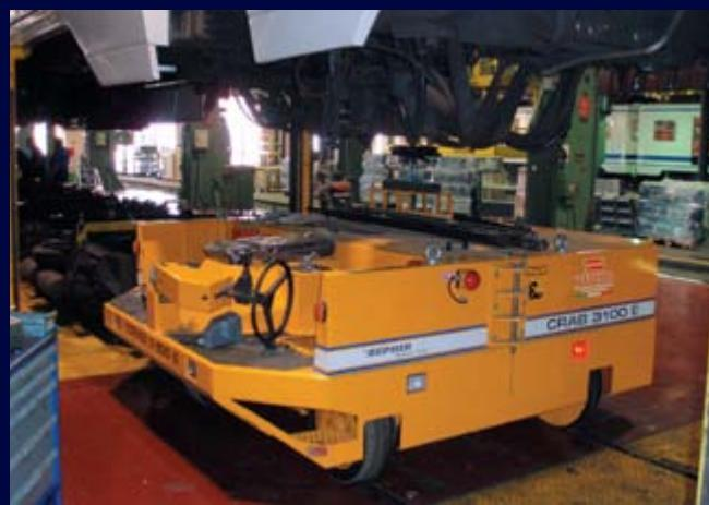
Low profile version for working as bogie mover under the lifted trains.
