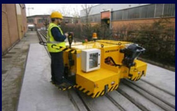
The most compact rail road battery operated shunter. Zephir patented design. Absolute minimum insertion width between rail vehicles and high manoeuvrability. Strong and robust construction for long life and heavy duty applications. The best researched investment, multipurpose logistic solution for each rail workshop. Perfectly designed for operation on the transfer bridge and for bogie handling.
